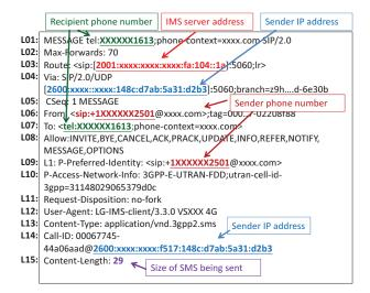
Figure 3: The SIP message header of an SMS message.
