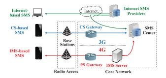
Figure 1: Architecture of the legacy (Internet-based and CS-based) and IMS-based SMS services.
