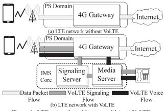
Figure 1: LTE network architecture with(out) VoLTE.
