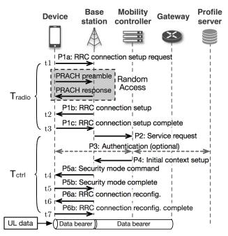
Fig. 4: Control-plane procedures for LTE data access
