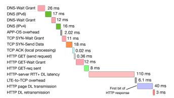
Fig. 6: Data access latency breakdown.
