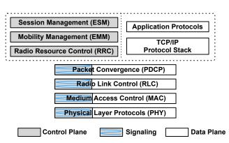
Fig. 2: LTE protocol stack for both control and data planes.
