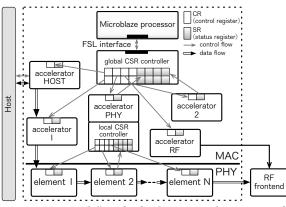
Figure 6: Control flow for both MAC and PHY in Tick.
