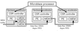
Figure 9: MAC layer accelerators architecture.
