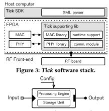
Figure 4: An *element* in *Tick*.
