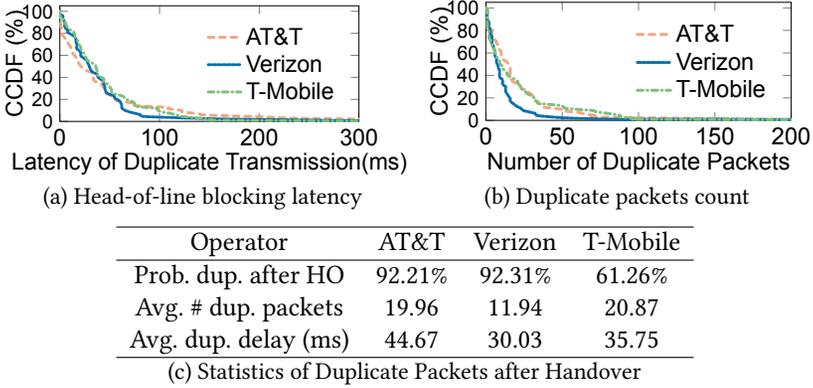
Fig. 7. HOL blocking of duplicate packets after handover.
