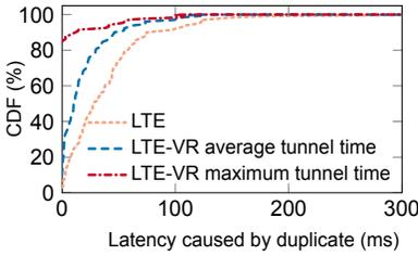
**Fig. 20. LTE-VR's savings for head-of-line blocking.**
