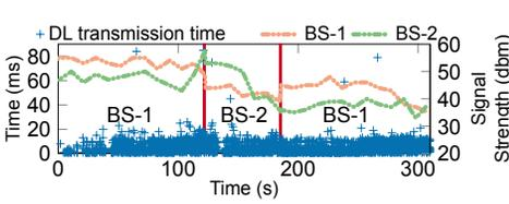
Fig. 15. A case of unnecessary handover.
