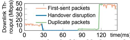
Fig. 10. Disruption & head-of-line blocking in handover.
