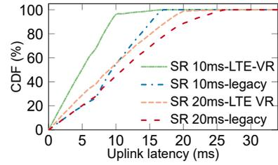
**Fig. 21. LTE-VR's uplink latency reduction.**
