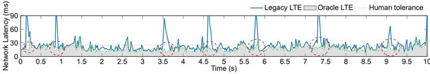
Fig. 2. Example of mobile VR’s network latency under good LTE signals (-90dBm).
