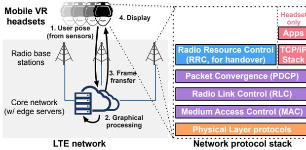
Fig. 1. Mobile VR over 4G (left); LTE network protocol stack (right).
