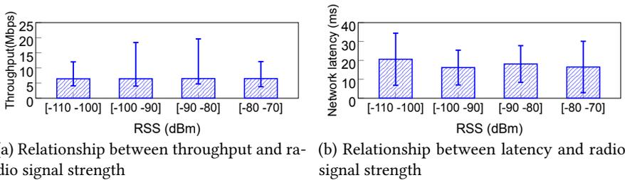
Fig. 23. Radio signal strength versus throughput/latency.
