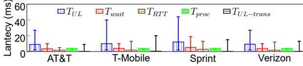
Fig. 11. Uplink latency breakdown in U.S. LTE operators.
